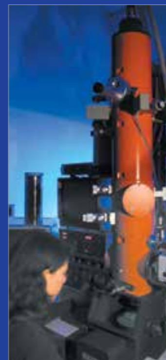
Transmission electron microscopy for studying the bulk morphologies of block copolymers.
