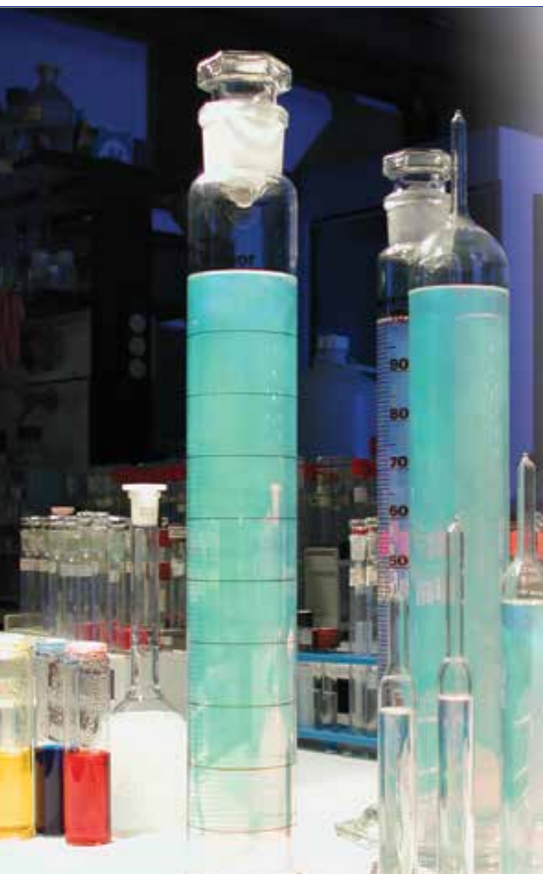
Typical particle size and spacing in colloidal solutions are in the range of the wavelength of visible light and therefore can lead to impressive colours, depending on the viewing angle.
