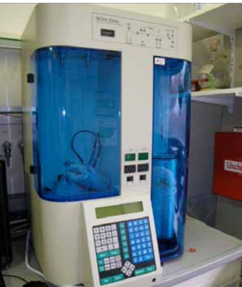
Nova 2000e - characterization of the porous heterogenous catalysts.
