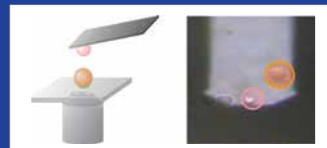
Measurement of the interaction forces between a pair of silica particles, which are immobilized on the cantilever and a glass substrate, respectively
