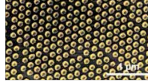
An array of crescent shaped gold nanoparticles obtained via nanosphere lithography.
