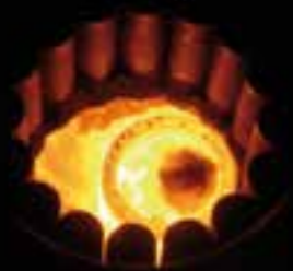
Skull Melting allows for crucible-free syntheses (part of the educts form the container) at a scale of ca. 200 grams and at temperatures up to 1750°C even at high oxygen fugacities.
