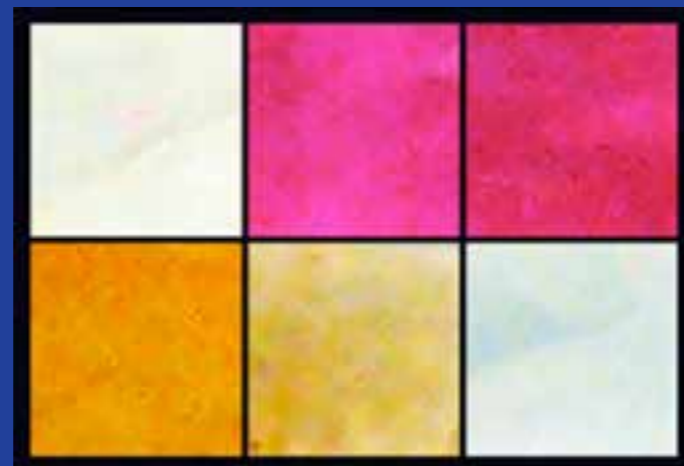
Chameleon nanofibers coated selectively with different dyes depending on the nature of the surface charges.
