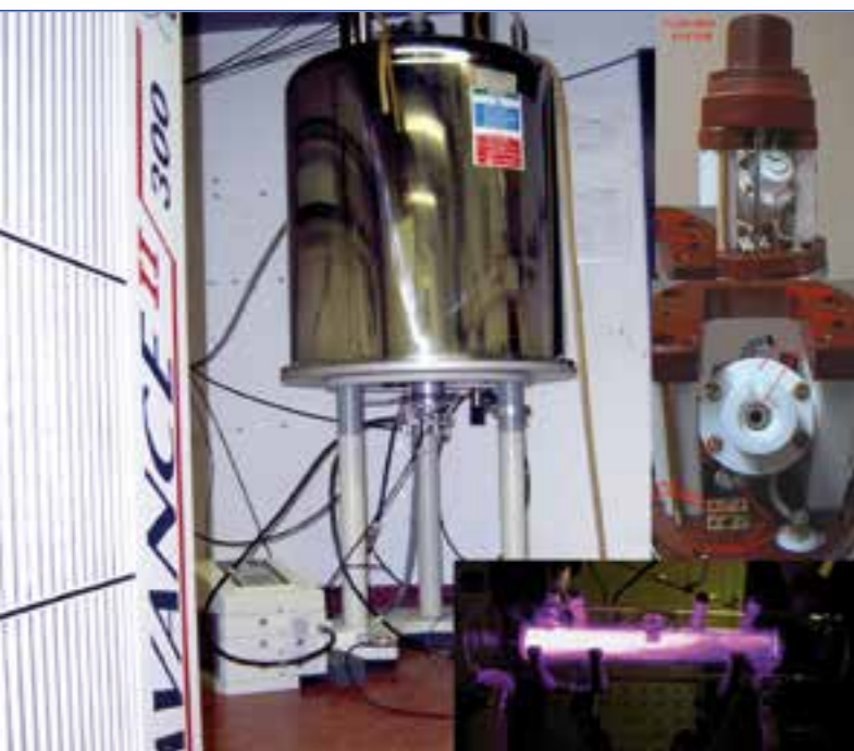
Solid-state NMR spectrometer including equipment for high-resolution measurements in crystalline and amorphous materials as well as surfaces and interfaces using hyperpolarized Xenon.
