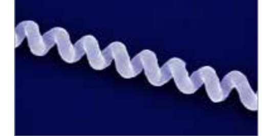
Polymer nanosprings obtained by electrospinning with complex electrode geometries.
