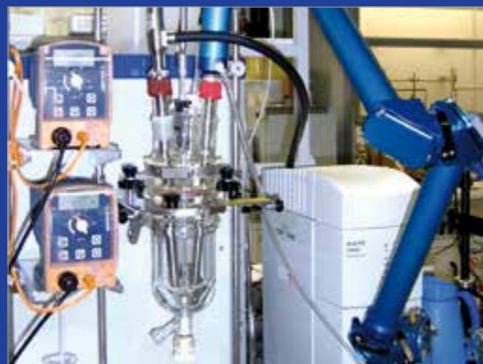
Automated laboratory reactor LabMax (Mettler-Toledo) equipped with IR- and FBRM probe (determination of particle size) allows for isolation of metastable polymorphs in microcrystalline form by controlling nucleation and growth.
