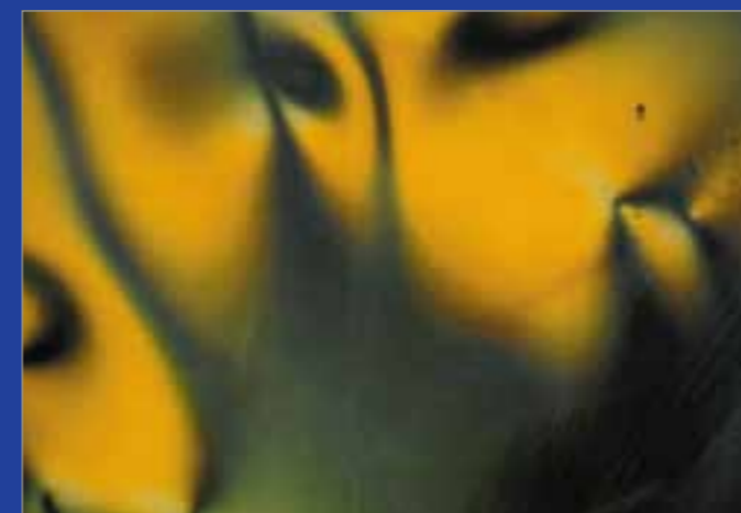
Micrograph by polarisation microscopy of a lyotropic liquid crystalline
